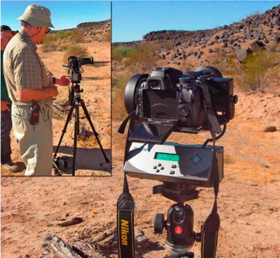
Figure 2. GigaPan robotic panhead in the field, Sears Point, Arizona, U.S.A. Photographs by Jennifer Huang.
